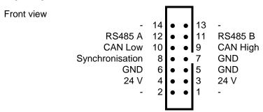
The ribbon cable connection is used to synchronise the detectors with each other and to provide the supply voltage and interface connection. The supply, synchronisation and interface connection to the control device can be made either using the ribbon cable or the backside DIN connector (see 7.3 Power supply).
