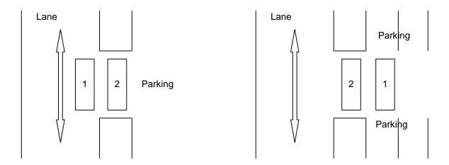
The placing of the loops depends on which travel direction backups are anticipated in. In travel direction 1  $\rightarrow$  2 no backups are permitted! In travel direction 2  $\rightarrow$  1 even vehicles in traffic line situations are correctly counted, whereby the vehicle gap must always enable a loop.
